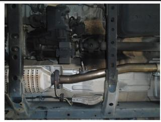
**Step 3:** Begin Installing the new system by attaching the inlet pipe to the Catalytic Converter outlet and attach the O2 sensor to the Inlet pipe, both with the removed OE Fasteners. **NOTE:** 96-00 4Runner's will use the longer inlet and 01-02 will use the shorter inlet.
