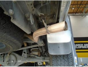
**Step 2:** Working front to rear, disengage all welded hangers from the rubber insulators and remove the system. (Retain the rubber insulators as they will be needed to mount the new MagnaFlow system.)
