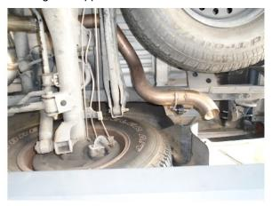
**Step 6:** Using the supplied rubber insulator and 2.50" clamp install the Tailpipe Assembly to the Muffler by fitting the hanger into the installed hanger bracket.
