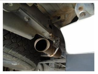
**Step 5:** Next, loosely attach the supplied Hanger Bracket Assembly to the underside of the P/S frame rail using the supplied fastener
