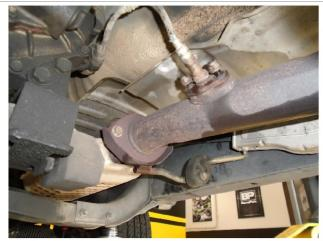
**Step 1:** To remove the OEM exhaust system, unfasten hardware at the muffler flange and remove the O2 sensor and secure out of the way (Retain both flange fasteners to be re-used).
